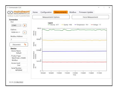
By selecting which graphs are displayed an operator can focus on one particular aspect and have an increased X-Axis.
